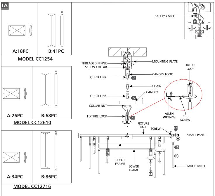
If necessary, screw the short end of the threaded nipple tightly onto the mounting plate, then screw the screw collar onto the threaded nipple.
